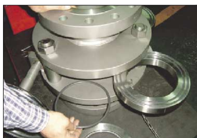
Step5. replace the internal O-ring
