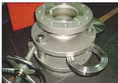
Step3. turn the spectacle plate 90 degree
