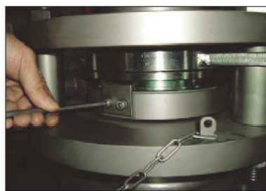
Step2. remove the both seat holder
