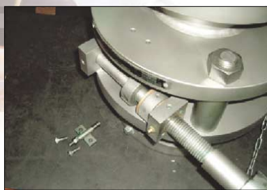
Step1. remove the position ass'y
